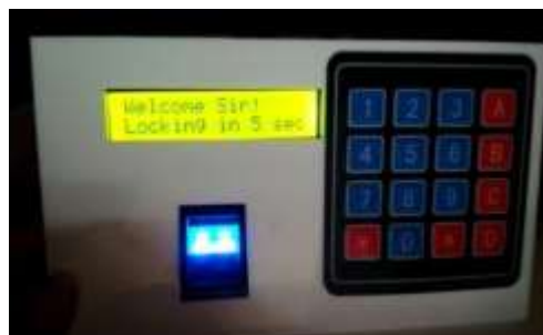
Fig 7. System displaying message after scanning fingerprint
